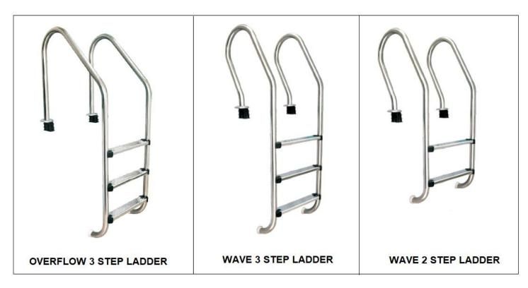
Stainless steel ladder with stainless steel steps made with trusted quality AISI 304 standard stainless steel with 1.1mm thickness. High resistance to corrosion with a shiny polished finish. The steps are also made of stainless steel with 500 mm width, safe and convenient to use with safety design to guard against slippage. The ladder comes with plastic stoppers that rest against the pool wall and protect it from damage and function as an anchor.
